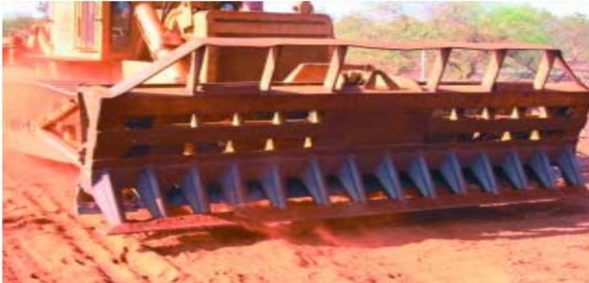
Figure 3-3 Mechanical rake for mesquite removal (Source: (Department of Natural Resources and Mines 2003)
